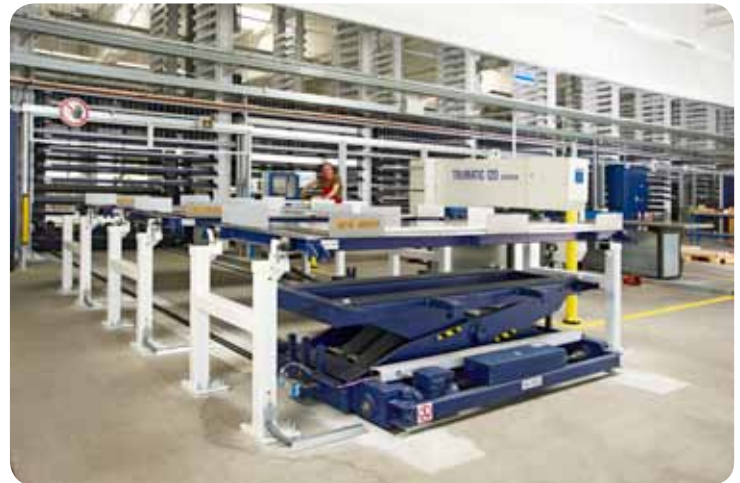
The three deposition frames buffer pallets with sheet stacks and thus ensure that the connected machine is fed. The scissors-type lifting platform can be lowered to pass underneath the pallets.
